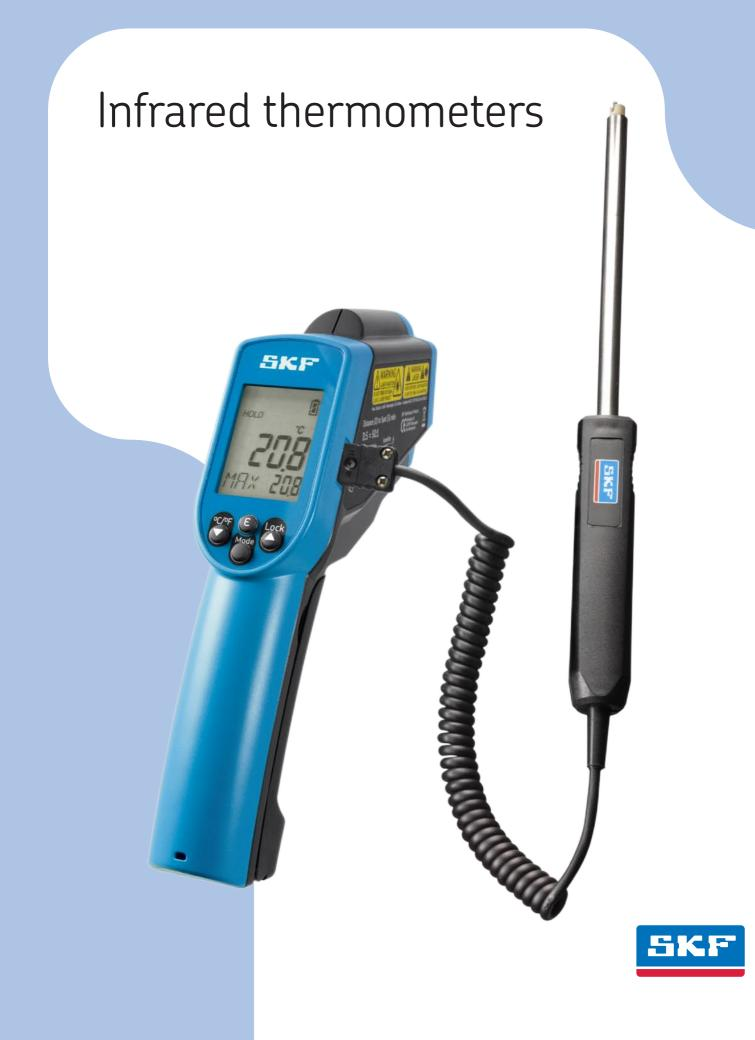
Infrared thermometers are portable, lightweight instruments for safely measuring temperature at a distance. They are extremely user-friendly; simply aim and pull the trigger and the temperature is shown on the display. These robust instruments are equipped with a back-lit display and laser sighting. They are fitted with a bright LED illuminator to allow the application object to be seen even in poorly lit environments.
