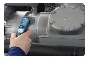
When used in non-contact mode, the thermometer senses the thermal energy radiated from an object with an infrared detector. When pointed at an object, the infrared detector collects energy, producing a signal that the microprocessor translates as a reading on the backlit display.
